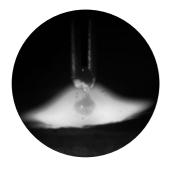
WIRE ORIENTATION **DOES NOT AFFECT ARC CHARACTERISTICS** IN CONTRARY TO **CONVENTIONAL TANDEM SOLUTIONS WITH TWO ARCS**
